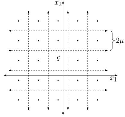
Fig. 1. Illustration of the quantizer for the two-dimensional state space,  $N = 5$ . The dashed lines define the boundaries of the quantization regions. The black dots define where the quantizer estimates the state to be, given the index of the quantization region that currently contains the state. Note that the quantizer output gives a displacement from  $\mathbf{c}$ .
